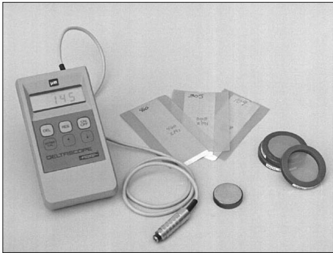
Figure 35. A magnetic induction thickness measuring device ("Deltascope") with mesh standards.
