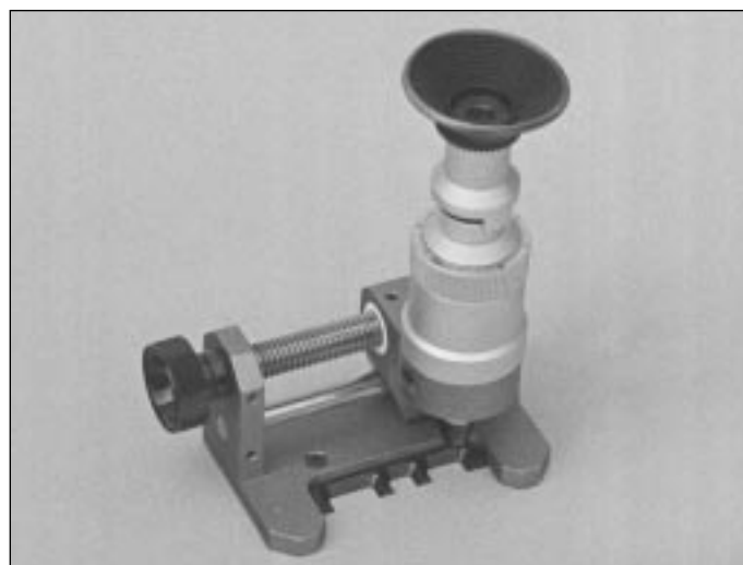
Figure 29. Tetko's Mesh Counter used for measuring mesh count in SPTF's research.
